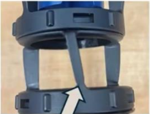
Visual demonstration of deformation
